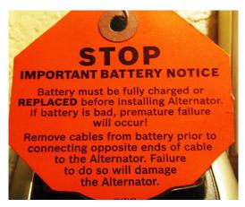
Replacement alternators for some newer cars will have a tag attached to them from the manufacturer or rebuilder as shown on the left. There is a reason for it.
