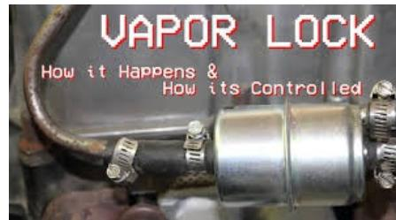
collapse of the fuel hose between the supply line and the fuel pump. This hose may have a flexible steel braid surrounding it to protect it from kinking, and also chafing against the frame of the vehicle.
